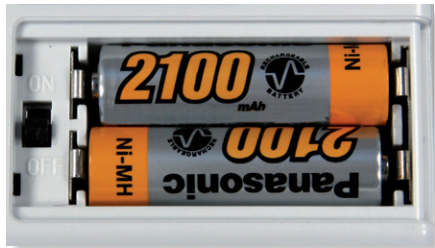
Operation with only 2 AA-size rechargeable batteries
