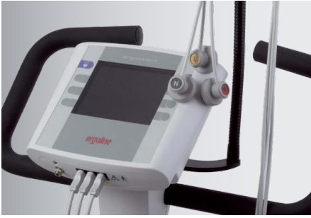
Electrode application system
